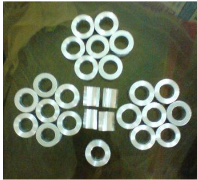
Figure1 Prepared workpiece samples from stir cast MMC ingot
