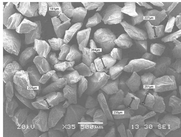
**FIGURE 2: SEM IMAGE OF SILICA QUARTZ PARTICLES AT 35X**
