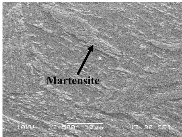
**FIGURE 4:** SEM IMAGE OF AISI 420 (MAG.2500X)
