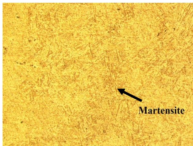
**FIGURE 7: OPTICAL METALLOGRAPH OF CA6NM (MAG.200X)**
