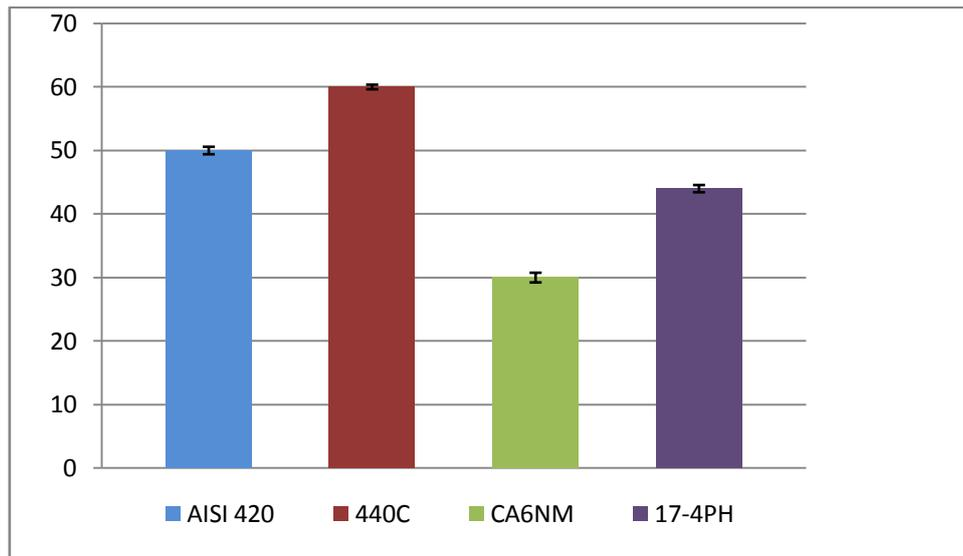
**FIGURE 10: HARDNESS VALUES AFTER HEAT TREATMENT**
