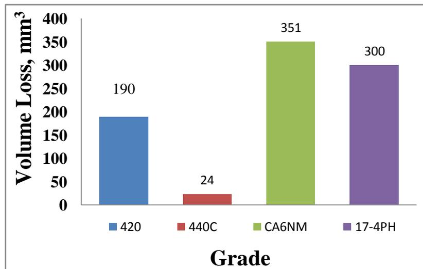
**FIGURE 11: VOLUME LOSS OF TESTED GRADES**
