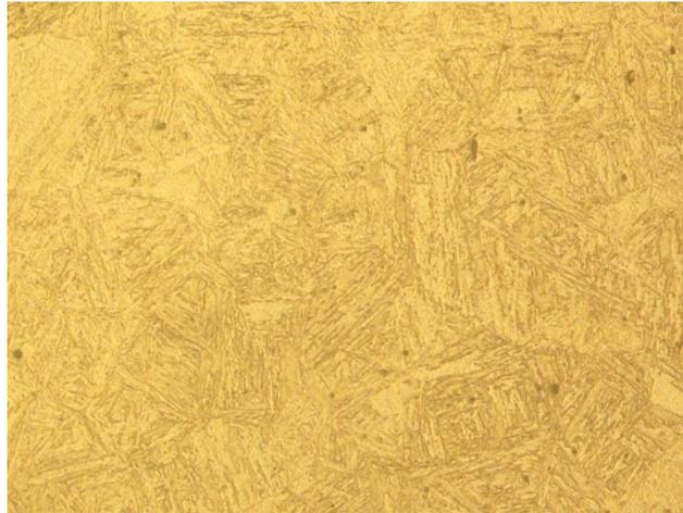
**FIGURE 3:** OPTICAL METALLOGRAPH OF AISI 420 (MAG.200X)
