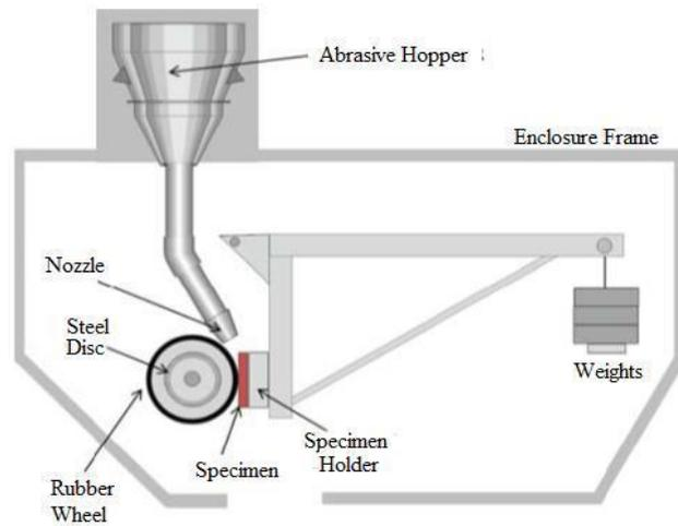
**FIGURE 1: SCHEMATIC OF DRY SAND/RUBBER WHEEL ABRASION TEST SET-UP**
