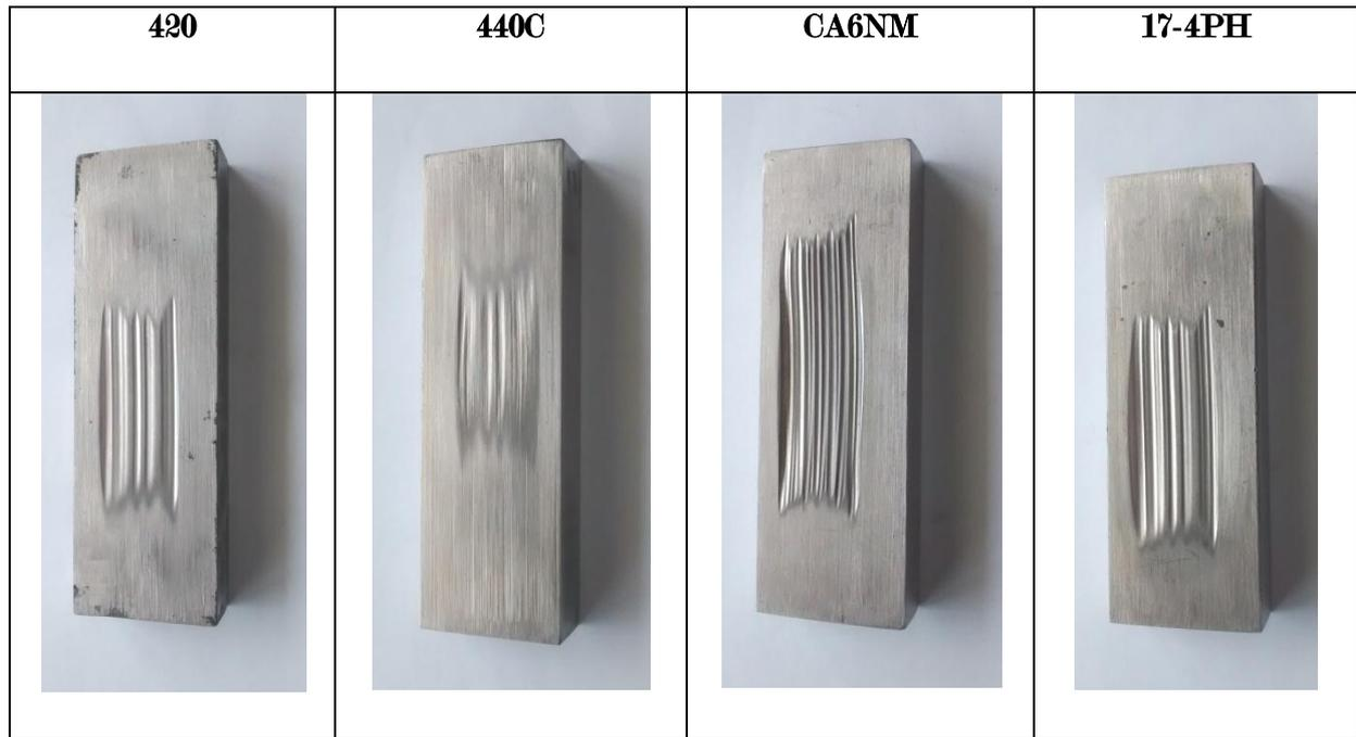
**FIGURE 12:** ABRASION WEAR PATTERN ON TESTED SAMPLE
