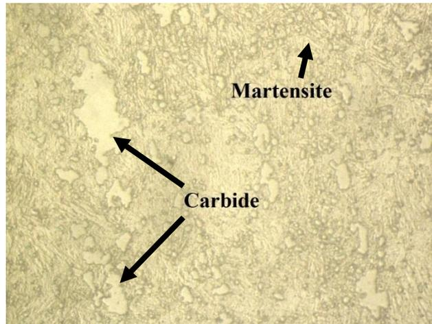
**FIGURE 5:** OPTICAL METALLOGRAPH OF AISI 440C (MAG.1000X)
