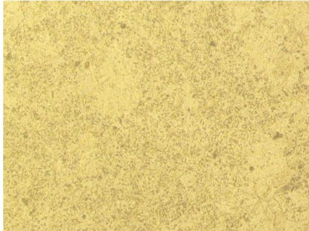
**FIGURE 8: OPTICAL METALLOGRAPH OF 17-4PH (MAG.200X)**
