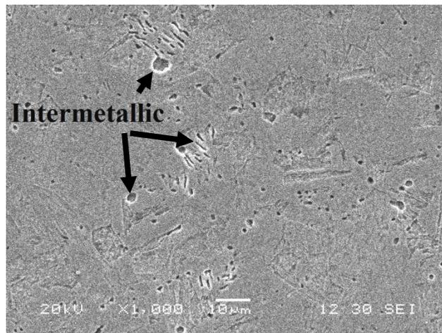
**FIGURE 9: SEM IMAGE OF 17-4PH (MAG.1000X)**
