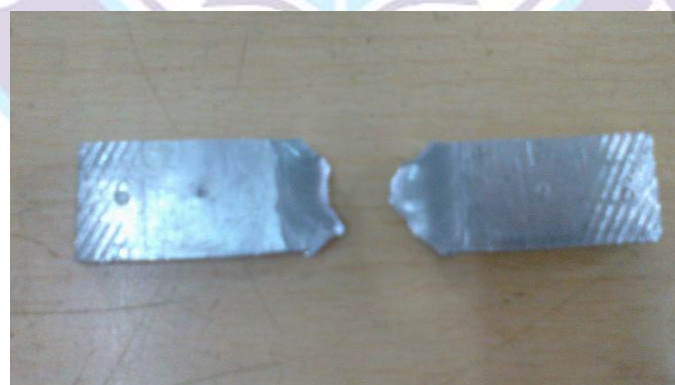
Specimen after failure under tensile testing
